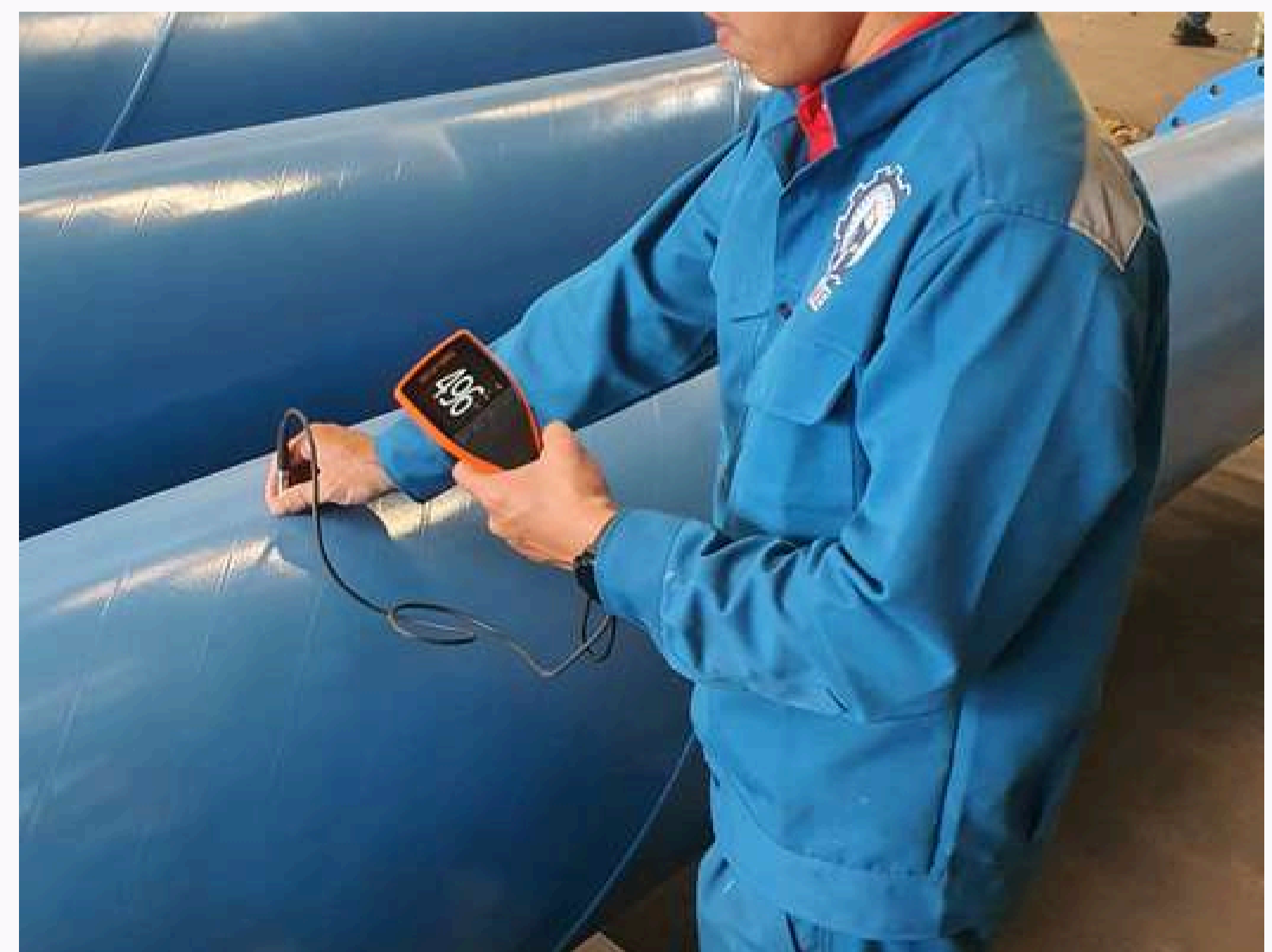
Dry Film Thickness Inspection
