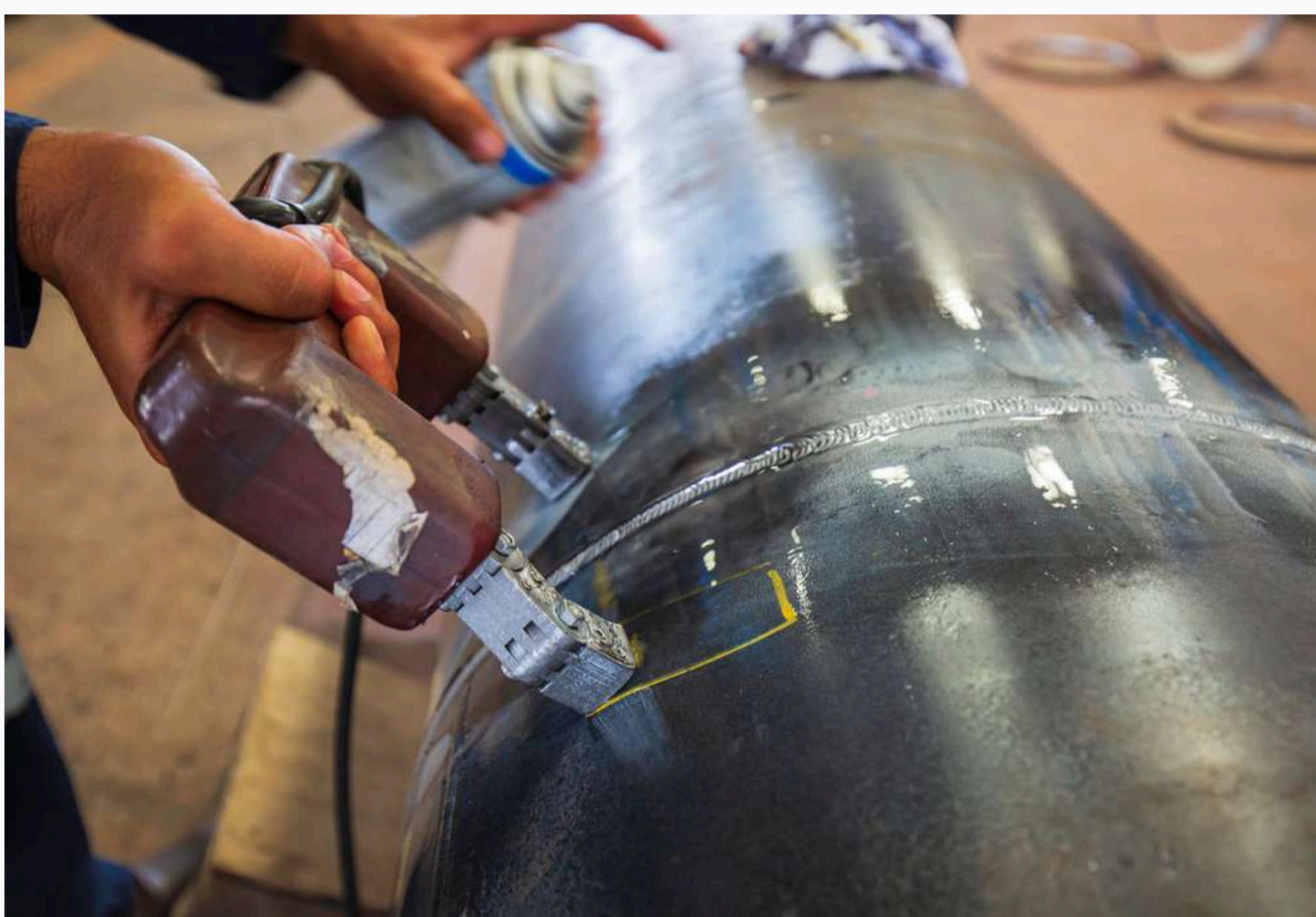
Magnetic Particle Inspection
